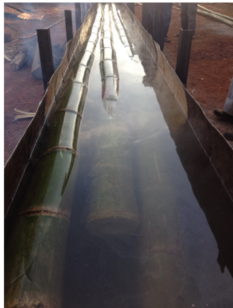
Bamboo soaking for 5 hours in heating solution
